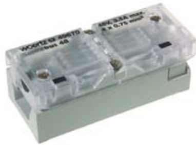
Connecting box for 2 round cables 4x0.75mm 2 flex with 1 connector and 3 contacts for supply and branching, specially adapted to MP bus devices from the company Belimo
